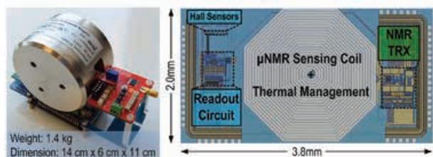
Fig. 1. The proposed NMR platform with magnetic field calibration and the chip micrograph.
