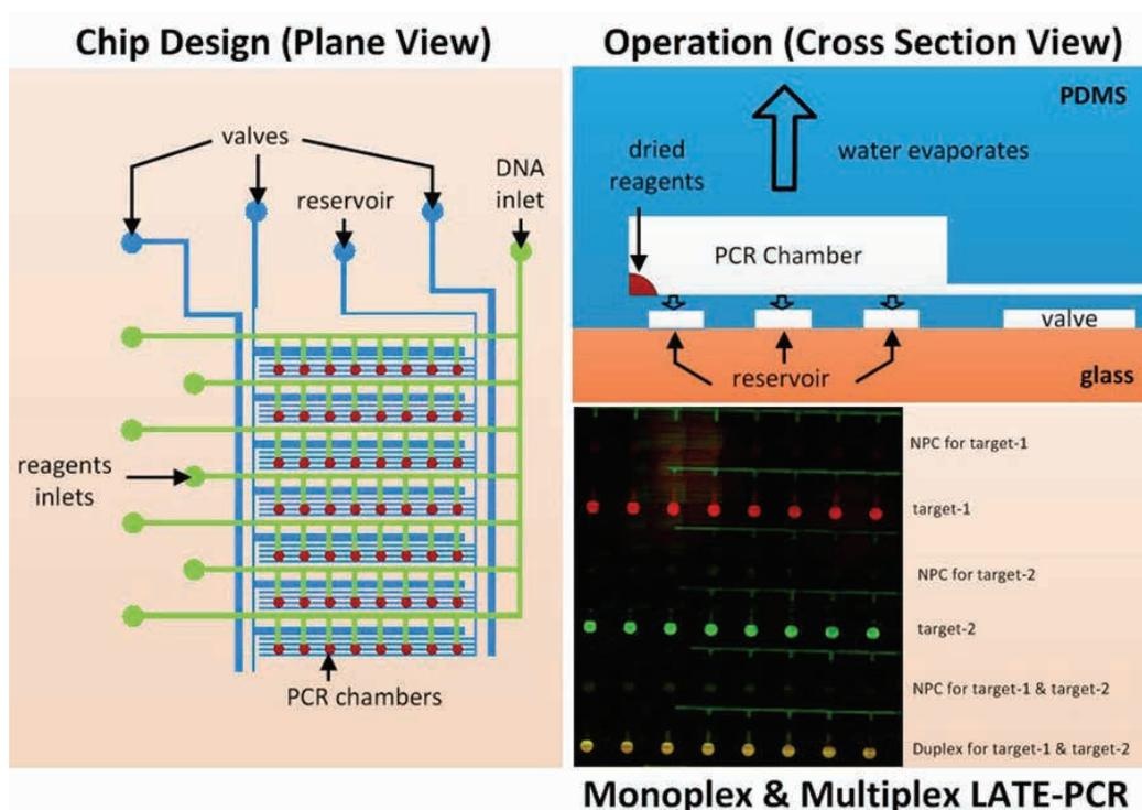
Fig. 1. preloading all of the reagents required for on-chip LATE-PCR amplification and detection of monoplex and multiplex single-stranded DNA products.
