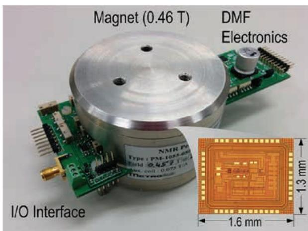
Fig. 1. The prototype of the platform and the fabricated CMOS NMR transceiver in 180nm process (inserted inside the magnet).
