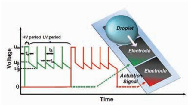
Fig. 1. Profiles of the electrode-driving signal, Natural Discharge after Pulse (NDAP), for a droplet moving across two electrodes. The high-voltage  $u_\alpha$  (HV) period lasts a period of  $t_\alpha$ . The low-voltage (LV) period includes multi-cycles of natural discharges ( $t_\beta$ ) and DC pulse ( $t_\alpha$ ).  $u_\beta$  is the instantly decreased voltage when disconnecting an electrode.  $u'$  is the lowest voltage to maintain the movement of a droplet.
