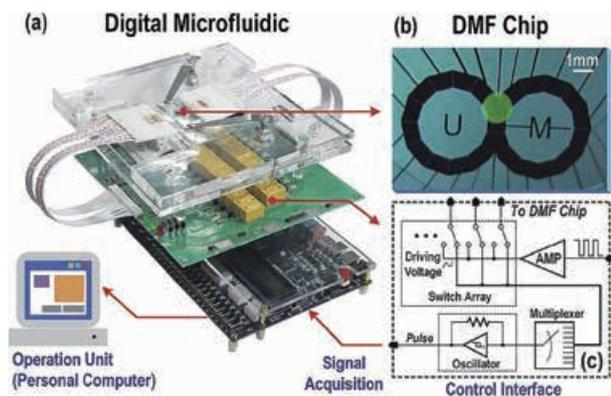
Fig. 1. Setup of the control-engaged DMF system.
