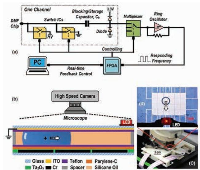
Fig. 2. Experimental setup for measuring the droplet dynamics under different electrode-driving signals.
