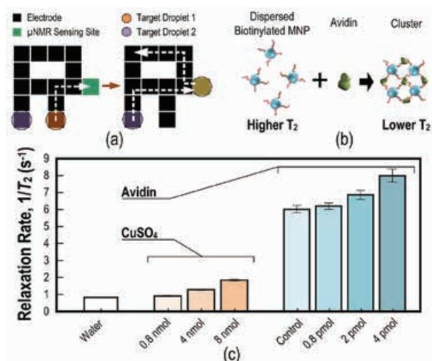
Fig. 2. (a) Multi-sample management scheme for the system. (b) Illustration of the sensing mechanism for avidin. (c) Relaxation rate ( $1/T_2$ ) from various targets.
