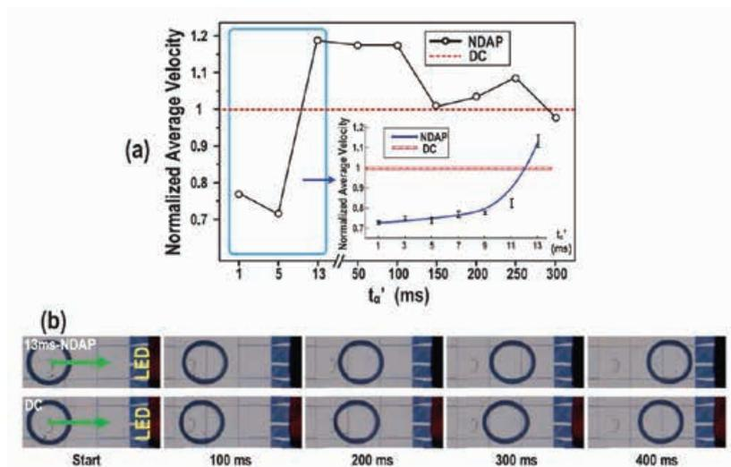
Fig. 2. (a) Normalized average velocity of a droplet under NDAP signals with different  $t_0$  and DC. Inserted curve shows the droplet velocities with  $t_0 < 13$  ms. The data were normalized at the average velocity under DC. (b) Video frames of a droplet actuated by NDAP and DC crossing 2 electrodes.
