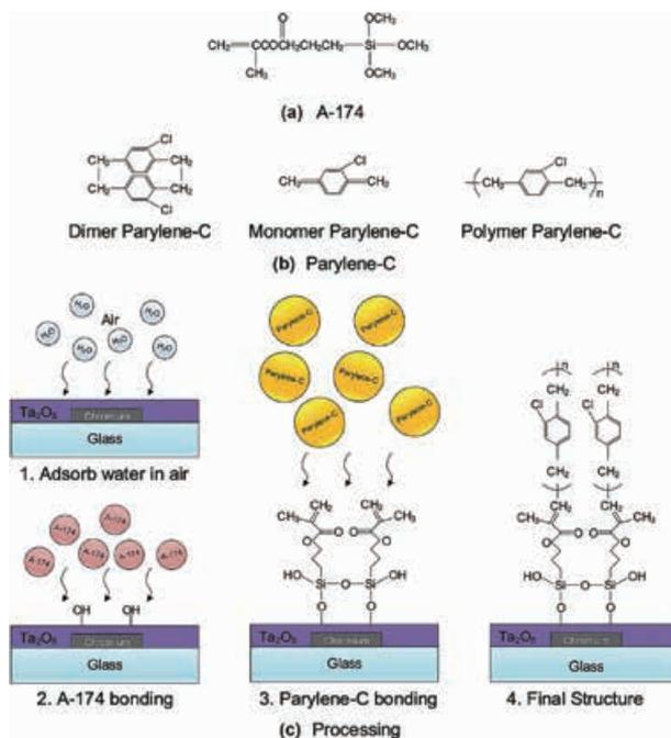
Fig. 2. Schematics of A-174 promoting adhesion between Ta<sub>2</sub>O<sub>5</sub> and Parylene C.
